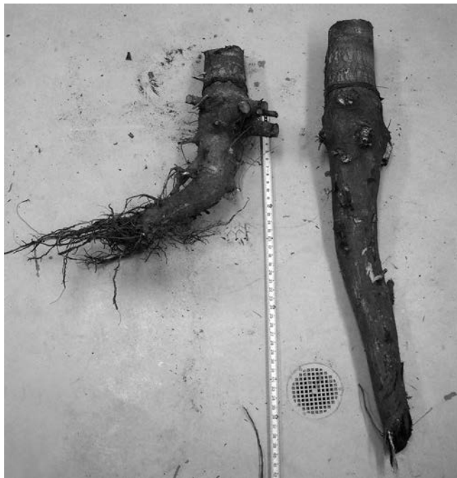
Figure 1. Taproot of ~15-cm diameter Torrey pine ( Pinus torreyana ) trees growing on (left) and off (right) a landfill liner. Note that the taproot of the tree on the liner turns abruptly left and splits into several smaller roots, whereas the taproot of the tree growing off the liner is straight.
